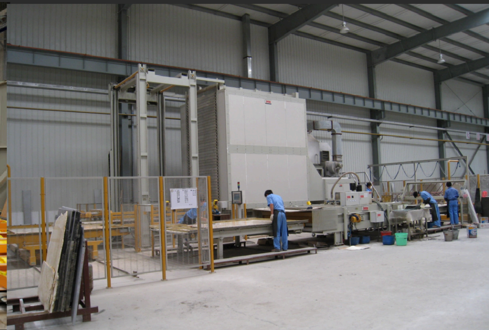
Vacuum Resin Lines
